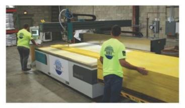
Now featuring full gasketing capabilities with our new Flow Water Jet CNC machine. Insulation cut to exact specifications for OEM, mechanical, and many other applications.
